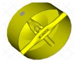
Figure 7: A LANL designed  $\beta$ =0.125 3-gap spoke resonator with RF-focusing in the center-gap.
