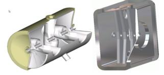
Figure 2: Multi-gap spoke resonators with cross- (left, ANL) and parallel (right, INFN-Legnaro) aligned spokes.
