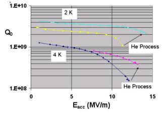
Figure 5: Test results for the LANL  $\beta$ =0.175, 2-gap spoke resonator.
