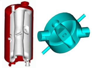
Figure 1: Simple coaxial (left, Argonne National Lab (ANL)) and spoke-type  $\lambda/2$  resonators (right, LANL)
