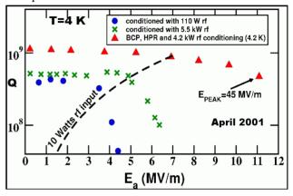
Figure 4: 4.2 K test results for the ANL  $\beta$ =0.4, 2-gap spoke resonator.
