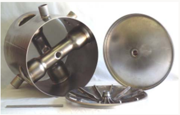
Figure 5A: Niobium elements of the 345 MHz double-spoke cavity prior to closure welds.
