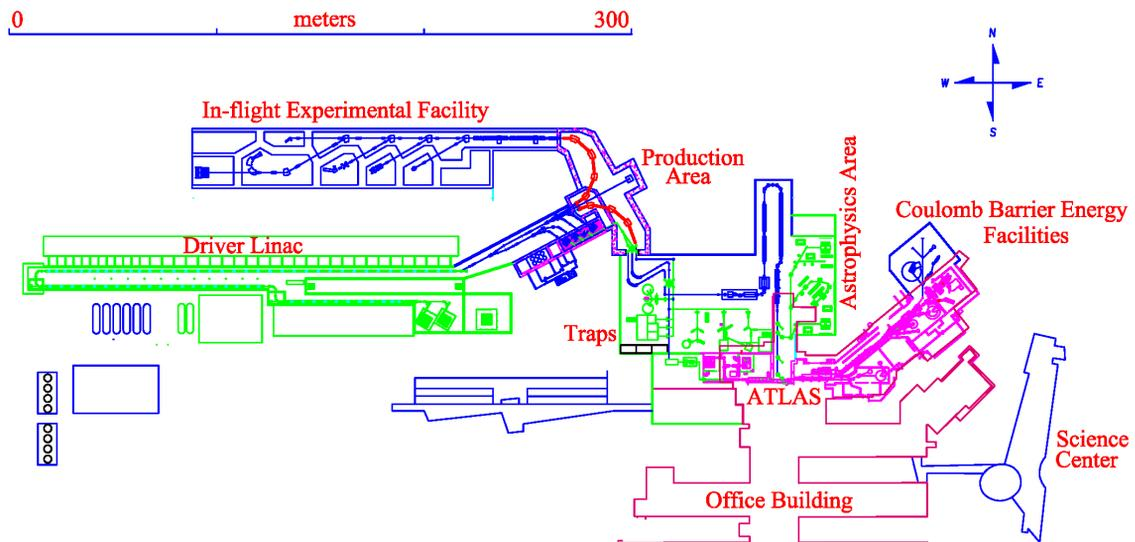
**Figure 2.** RIA layout proposed by Argonne National Laboratory (ANL).
