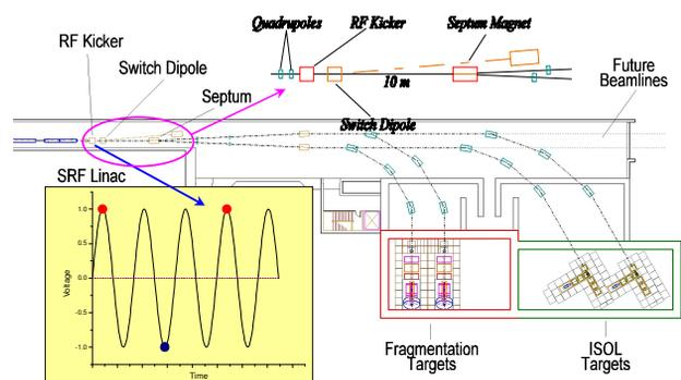
**Figure 9.** Schematic layout for distribution of stable isotopes accelerated in the driver linac to the radioactive beam production targets.
