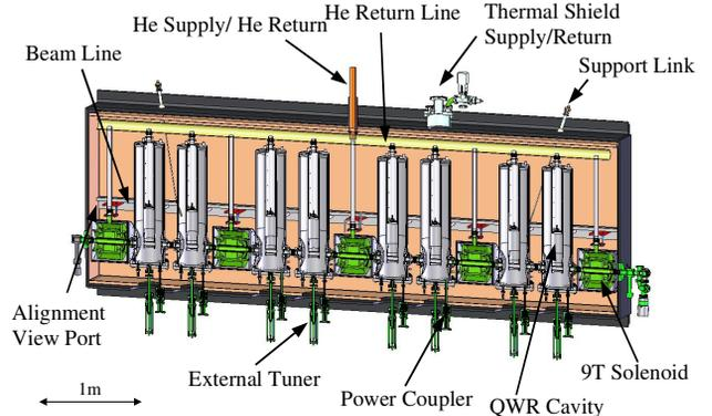
Figure 6. RIA cryomodule concept for  $\lambda/4$  and  $\lambda/2$  cavity geometries.
