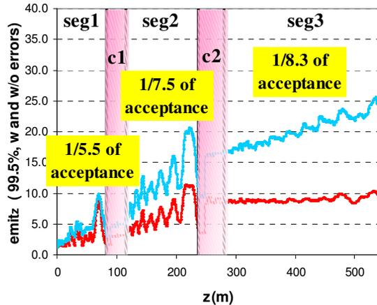
**Figure 7.** End-to-end simulation of the RIA driver linac for the longitudinal phase space. The first, second, and third linac segments are labeled seg1, seg2 and seg3, while the two charge-stripping regions are labeled c1 and c2. The results for the case of no errors are shown in red. The worst result for any of 100 seeds at each longitudinal position is plotted in blue.
