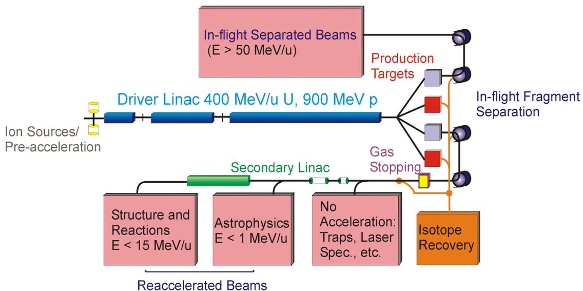
**Figure 1.** Conceptual layout of the Rare Isotope Accelerator (RIA) facility.
