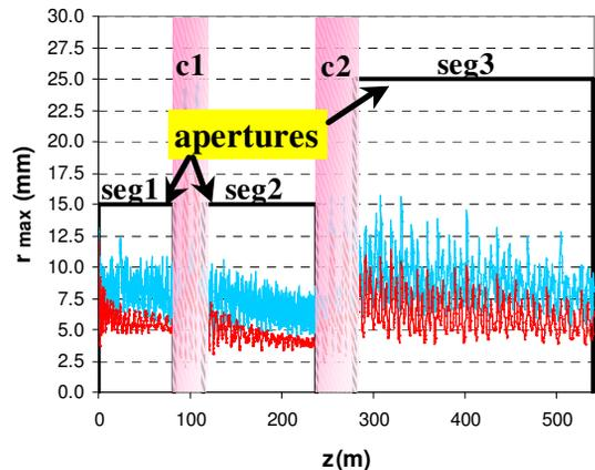
**Figure 8.** End-to-end simulation of the RIA driver linac for the transverse phase space. The results for the case of no errors are shown in red. The worst result for any of 100 seeds at each longitudinal position is plotted in blue.
