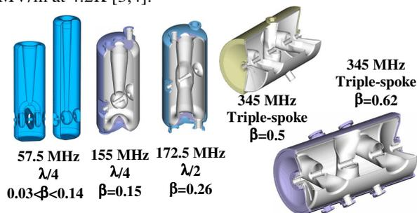
**Figure 3.** Six cavity types for the ANL RIA driver linac.
