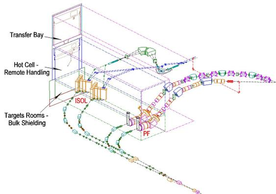
**Figure 10.** Schematic layout of the RIA radioactive beam production target area.
