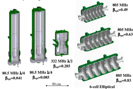
Figure 5. Six cavity types for the MSU RIA driver linac.
