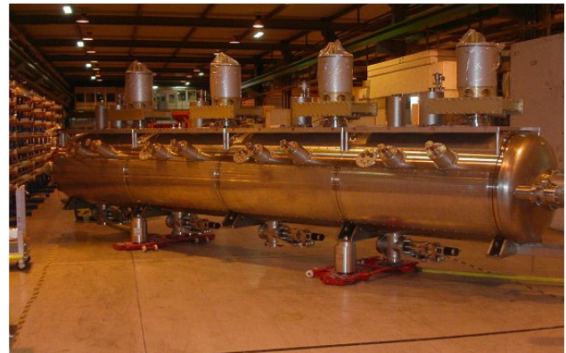
Figure 8: LHC module housing 4 single cell cavities operating at 400 MHz
