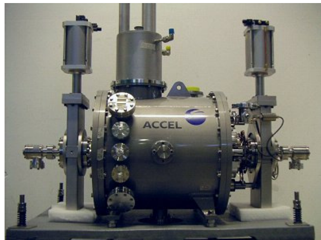
Figure 11: Higher harmonic cryomodule for BESSY
