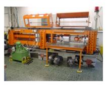
Figure 2: The hydroforming machine.
