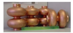
Figure 4: Double cell NbCu clad cavities recently produced at DESY from KEK tubes (no cracks on the inside surface).
