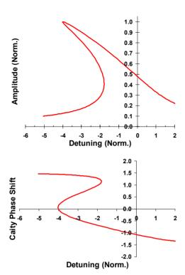
Figure 2: Resonance curve and phase shift across a cavity when driven by a fixed-frequency source in the presence of ponderomotive effects.
