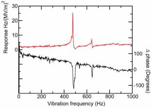
Figure 1: Lorentz transfer function of a  $\beta$ =0.61, 805 MHz 6-cell elliptical cavity (top) [10], and of a double-spoke 352 MHz,  $\beta$ =0.4 cavity (bottom) [11].
