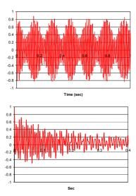
Figure 7: Examples of autocorrelation function of frequency fluctuations measured on SNS cavities. At the top microphonics are generated by 2 single-frequency sources; below they are generated by broad-band noise.
