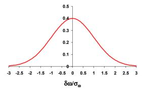
Figure 4: Probability density of cavity frequency fluctuations  $\delta \omega_{ex}$  generated by a sinusoidal (top) or gaussian white noise (bottom) external disturbance n(t).
