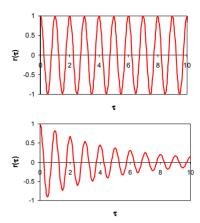
Figure 6: Normalized autocorrelation function of the output of a harmonic oscillator when driven by a sinusoidal input (top) and gaussian white noise (bottom).
