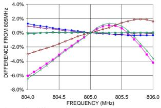
Figure 13: Difference between RF power measurements calibrated at 805 MHz and those taken at nearby frequencies for several different signal paths.
