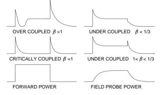
Figure 14: Upper four traces are depictions of reflected power waveforms for various coupling states. The lower two traces are the corresponding forward and field probe pulse shapes.
