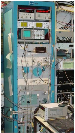
Figure 6: Example of a research and development system which is capable of being operated at frequencies between 500 MHz and 3 GHz.
