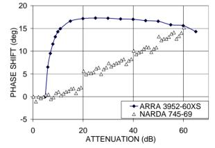
Figure 2: Phase shift as a function of attenuation for two different mechanical attenuators.
