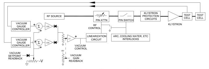
Figure 9: Block diagram of a vacuum conditioning system.
