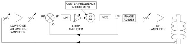
Figure 1: Block diagram of a typical VCO-PLL system which includes an RF amplifier and cavity structure.
