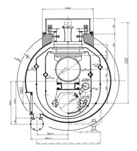
Figure 4 cross-section of STF Phase 1 cryomodule
