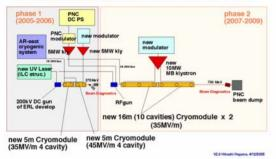
Figure 1 STF accelerator block-diagram. Phase 1 plan and Phase 2 plan are shown in each square block.
