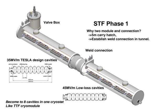
Figure 5 STF phase 1 connected-cryomodule.
