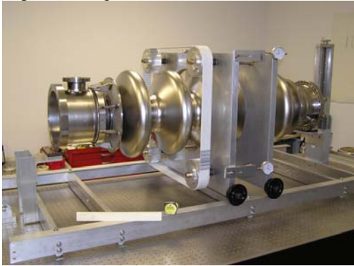
Fig. 3. The BNL niobium cavity being tuned.
