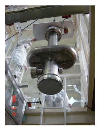
Figure 7: High pressure rinsing; KEKB crab cavity #2 with transition flange under high pressure rinsing.
