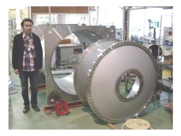
Figure 13: Vacuum vessel for KEKB crab cavity.
