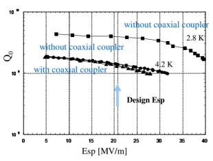
Figure 5: Measured  $Q_0$  of KEKB crab cavity #1 without and with coaxial coupler.
