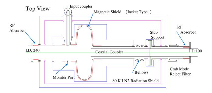
Figure 8: Conceptual design of the KEKB crab cavity in the horizontal cryostat.
