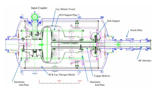
Figure 10: Detailed design of the KEKB crab cavity (Top view).
