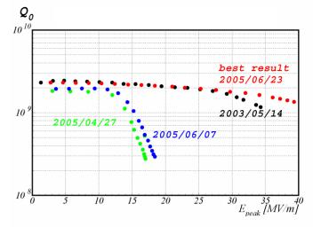
Figure 6: Measured  $Q_0$  of KEKB crab cavity #2.
