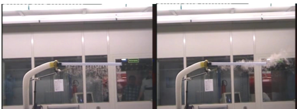
Fig. 3: Influence on laminar flow conditions during fan unit shut down. left: regular laminar flow - right: one fan unit switch off causes horizontal flow in class 100 area
