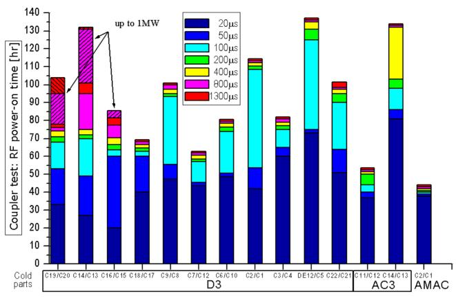
Figure 3: Couplers conditioning times: TTF3 and AMAC.
