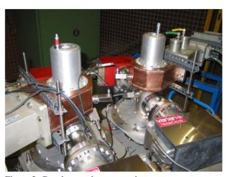
Figure 2: Couplers on the test stand.
