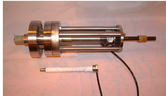
Figure 5: The piezoelectric fast tuner assembly used during the cavity tests and the piezoelectric actuator.
