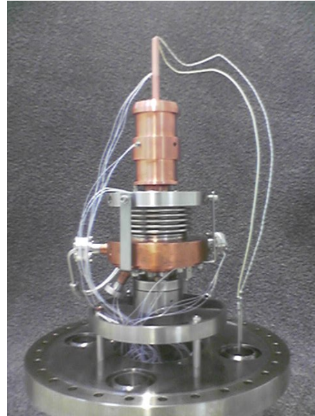
Fig.3: Photocathode cooling test-bench with temperature sensors and electrical heater on the top
