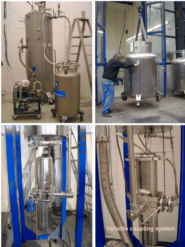
Figure 2: Vertical test facility at ACCEL. The cryostat (top left) is filled with helium out of dewars (top right). The superconducting half-wave resonator is equipped with a variable input coupler for the vertical test (bottom).
