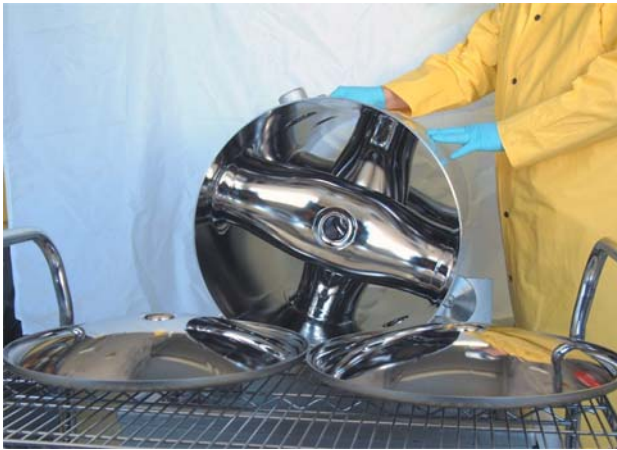
Figure 2: Major niobium subassemblies of the \beta=0.62 triple-spoke resonator after final electropolishing
