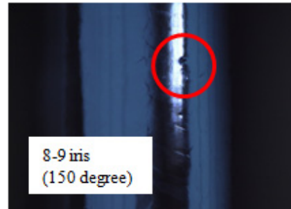
Figure 11: Inspection of cavity inner surface. A tip was found at iris between 8-cell and 9-cell.
