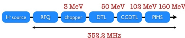
Figure 3: Block diagram of Linac4.
