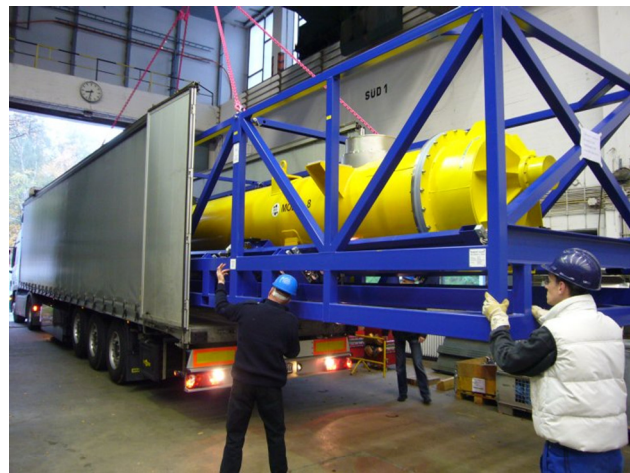
Figure 8: The first accelerator module on its travel from CEA Saclay / IRFU, Paris to DESY, Hamburg.
