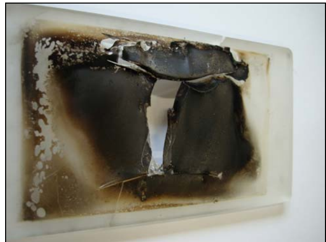
Figure 9: Booster cavity 2 (BC2) warm window failure.
