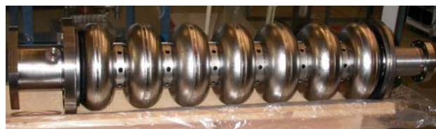
Figure 13: 7-cell cavity after final electron-beam welding.
