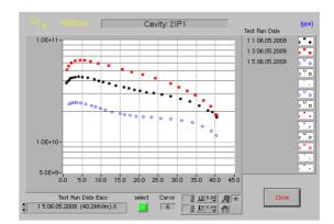
Figure 2: Pi modes of 2-cell cavity at 1.6, 1.8 and 2.0K.
