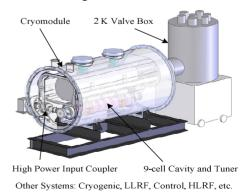
Figure 9: The cryomodule of 1.3 GHz 9-cell Nb as test stand.
