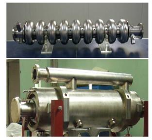
Figure 4: The 9-cell cavity of fine Nb grain with end groups in a Liquid He tank.
