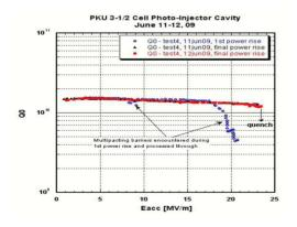
Figure 7: RF Test of 3.5 cell cavity at J-Lab.
