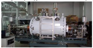
Figure 8: 500 MHz KEKB type SRF cavity for IHEP.
