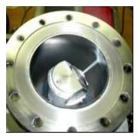
Figure 7: Nozzle of the dry ice cleaning apparatus.
