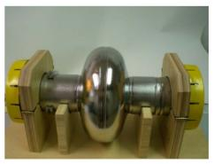
Figure 6: Single crystal Niobium cavity.
