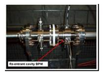
Figure 4: New re-entrant cavity beam monitor for XFEL
