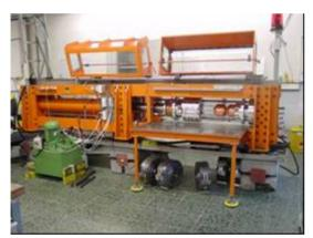
Figure 5: Hydro-forming apparatus for the production of seamless Niobium cavities
