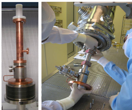
Figure 10: RF power coupler.
