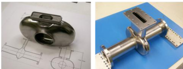
Figure 3: The proposed ANL crab cavity showing the on-cell damping waveguide.
