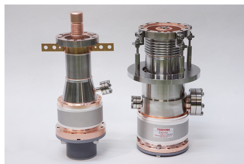
Figure 13: A set of a cold window part and a warm window part in the completed STF-II input coupler.
