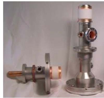
Figure 7: The TTF-V input coupler from LAL-Orsay.
