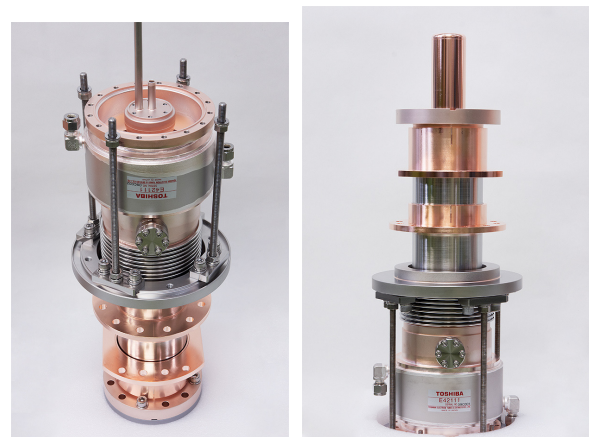
Figure 16: A completed cERL injector input coupler for a cw operation.
