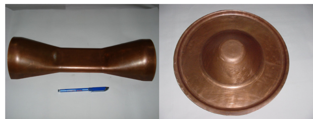
Figure 10: (a) Left – Half spoke formed in copper and after machining the edges & ends. (b) Right – End wall formed in copper. The edge has not been machined.
