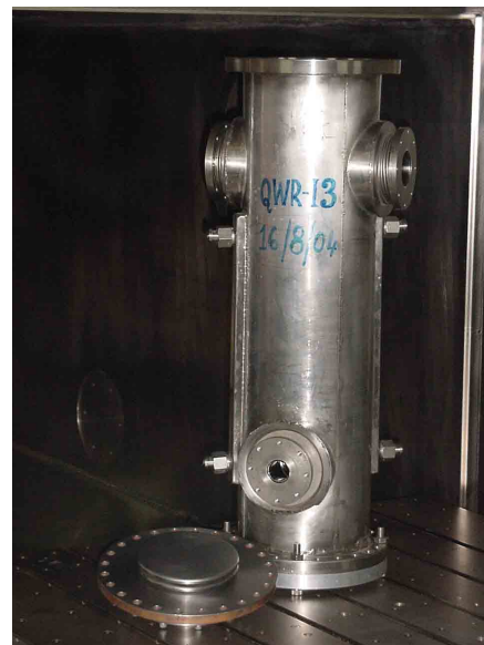
Figure 4: A completely indigenously fabricated QWR along with its slow tuner bellows.
