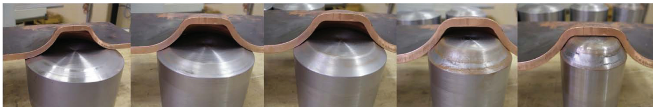
Figure 4: Progressive formation of the beam ports by deepdrawing on a test piece. The punches and die are changed for each step. A flame annealing of the copper is performed before each step, in order to soften it and prepare it for the deepdrawing.
