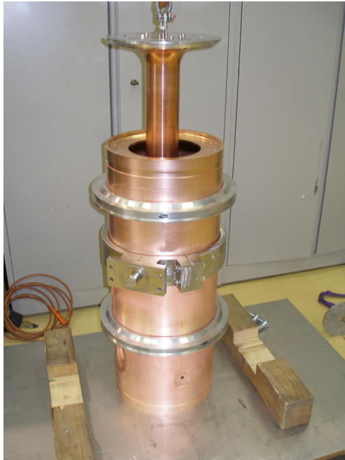
Figure 6: Mechanical assembly of cavity sub components for an intermediate RF check. This operation, as well as metrology controls, are carried out in a temperature-controlled room in order to ensure the best accuracy.
