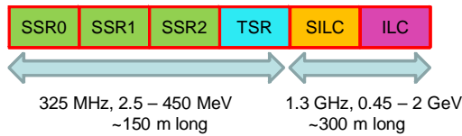
Figure 2: The schematic of the CW linac (2.5 MeV – 2 GeV).
