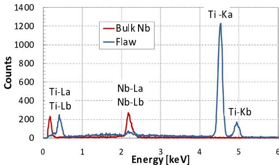
Figure 5: SEM analysis in the center of the groove and just aside it: while the defect is nearly full Ti, the material around the flaw looks unaffected by the welding failure (within SEM resolution limits).
