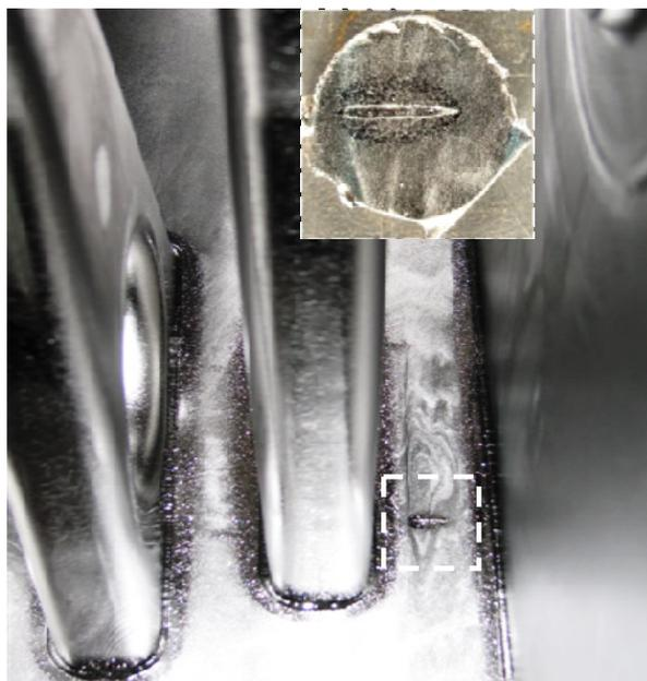
Figure 3: Photo of the Ti defect in the resonator (detail: the portion of Nb wall removed during the repair).
