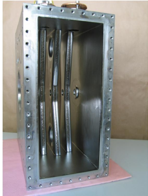
Figure 1: Photo of the ladder resonator prototype.
