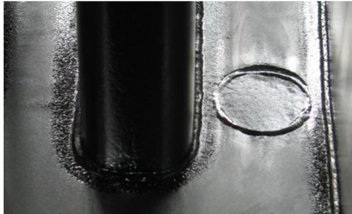
Figure 6: Completed repair of the EB weld flaw.
