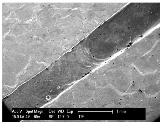
Figure 4: SEM picture of a portion of the defect: the darker part in the groove is titanium.
