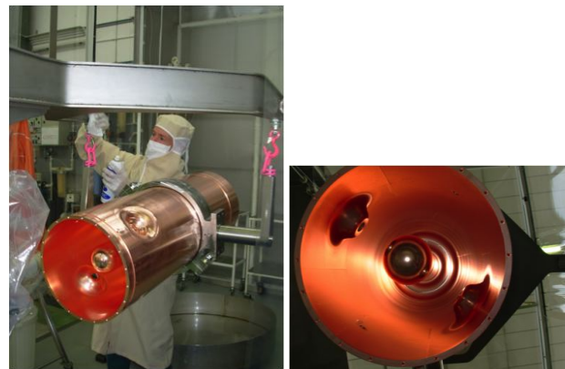
(a) the cavity during the cleaning process (b) internal view of the cavity
