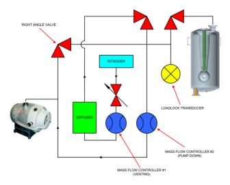
Figure 1: "Up-to-air" system schematic.
