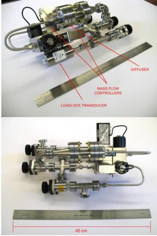
Figure 4: Assembled "up-to-air" system.
