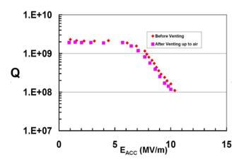
Figure 5: Plot showing Q-curve data from a single cavity test before and after the clean cavity space was vented and evacuated using the "up-to-air" system.
