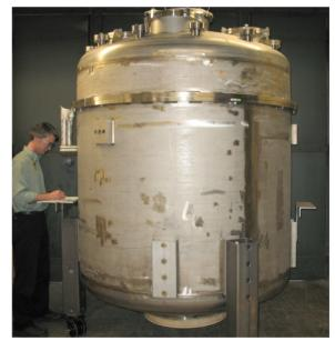
Figure 1: SRF Test Cryostat.
