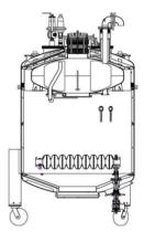
Figure 7: 9 cell elliptical cavity in TC3<sup>.</sup>
