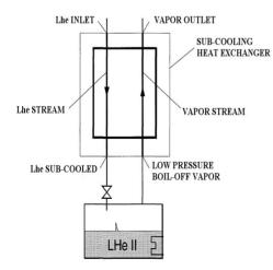
Figure 5: Heat exchanger flow schematic.
