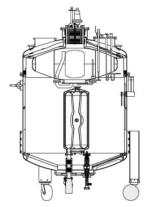
Figure 6: Half wave cavity in TC3<sup>.</sup>
