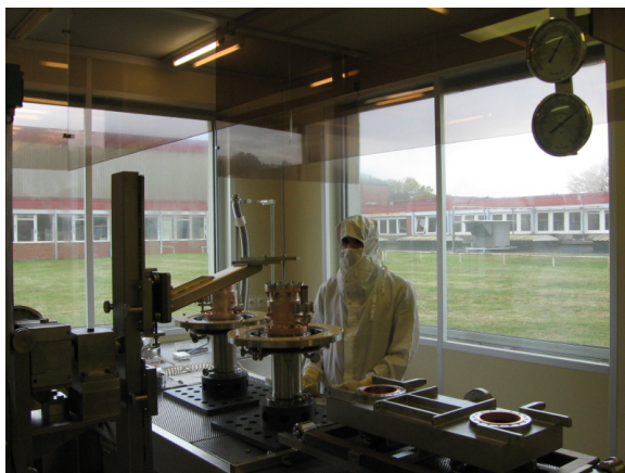
Figure 4: coupler assembly in the class 10 clean room
