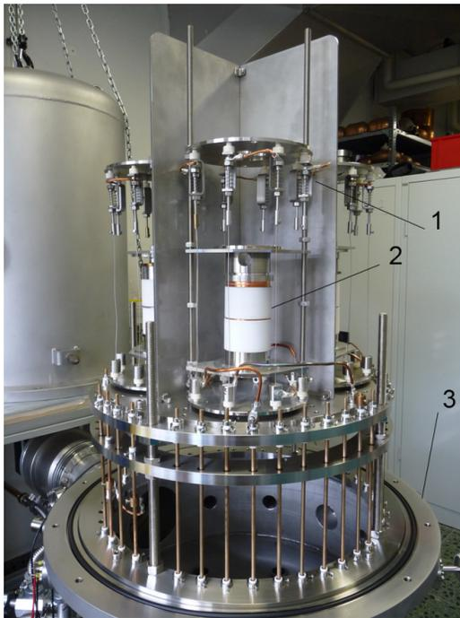
Figure 3: Inner assembly, with 4 mounted ceramics. 1: flexible suspension of the wire, 2: ceramic, 3: vessel flange.
