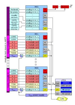
Figure 1: Block diagram of the interlock configuration for a module test stand in AMTF.
