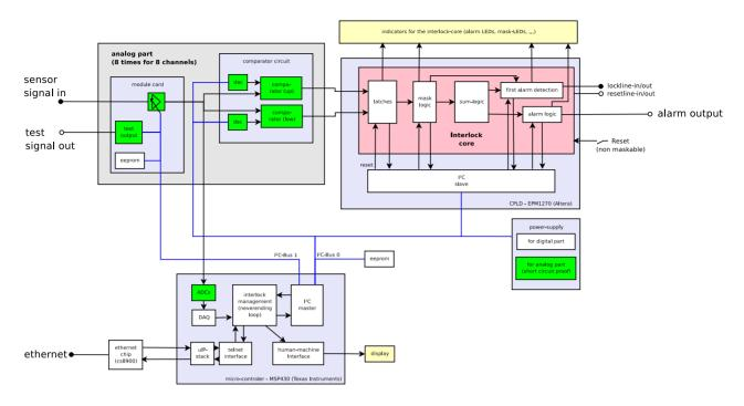
Figure 3: Block diagram of the interlock.
