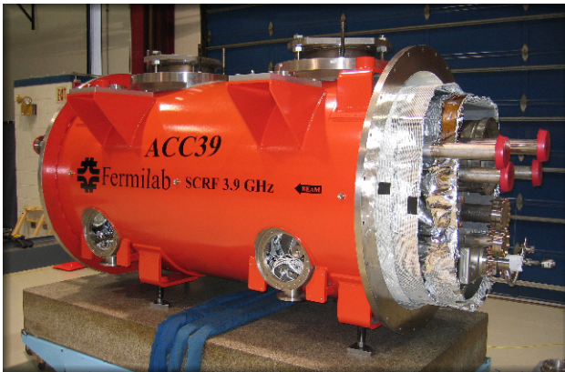
Figure 7: Recently Completed 3 rd Harmonic Cryomodule.
