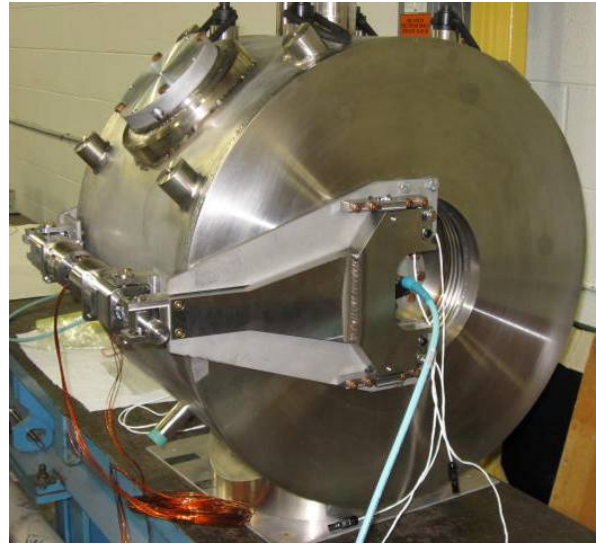
Figure 2: SSR1 cavity dressed into helium vessel with 2 tuners installed on both sides of vessel.
