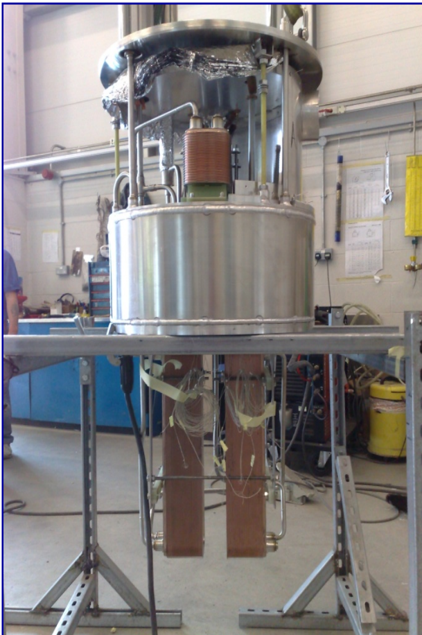
Figure 6: COOL-IT heat exchanger during assembly.
