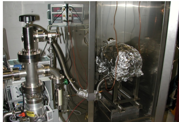
Figure 3: Test box with two pre-compressed windows ready to be baked under vacuum.
