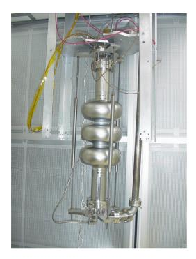
Figure 4: 3-cell cavity attached to test stand with external support rods. The cavity is located in the clean room in front of a horizontal laminar flow system.
