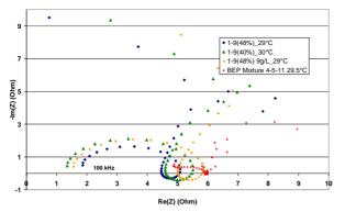
Figure 4: EIS Nyquist spectra obtained for different EP and BEP electrolytes at 4.5V Vs Ag/AgCl. Range 100 kHz -0.1 Hz. BEP differs significantly from EP.
