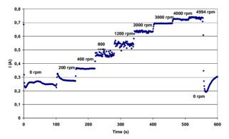
Figure 3a: I(t) obtained at 5V Vs Ag/AgCl with BEP for different rotation speeds. T=30  $^{\circ}$ C. Intensity increases with electrolyte's agitation.
