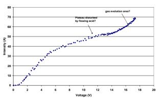
Figure 7: I(V) curve plotted on single-cell rotating CEBAF cavity. T=20 °C. 1 rpm. No clear plateau is observed.
