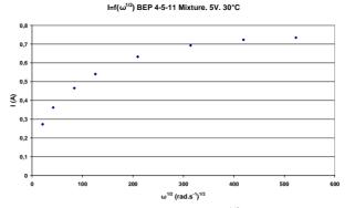
Figure 3b: Intensity as a function of  $\omega^{1/2}$  for BEP mixture. T=30 C. No proportionality is found. The electrochemical system is not governed by diffusion of fluorine.
