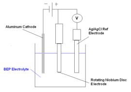
Figure 1: Set-up used for voltamperemetric measurements with rotating working electrode (niobium anode).
