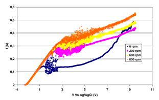
Figure 2: I(V) curves for BEP mixture plotted with a niobium rotating disc electrode at different rotation speeds. T=30 C.
