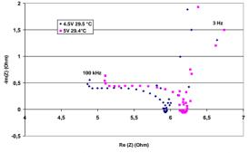
Figure 5: EIS Nyquist Spectra for BEP at 4.5 and 5 V Vs Ag/AgCl. Limit R0 at high frequencies increases with potential.
