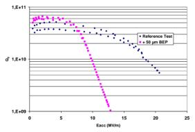
Figure 8:  $Q_0=f(Eacc)$  for C1-22 Tesla Shape cavity. Performances deteriorated after BEP with early Q-Slope.
