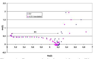
Figure 6: Features obtained at 4.5 and 5V are superimposable. (Range 100 kHz - 3 Hz).
