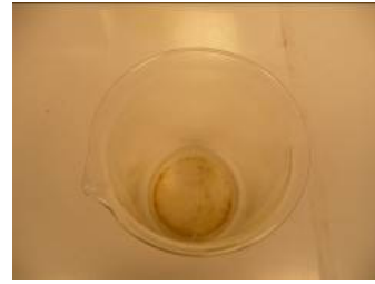
Fig. 7: Impurities are found in the chloroform used for several cavity rinsings.
