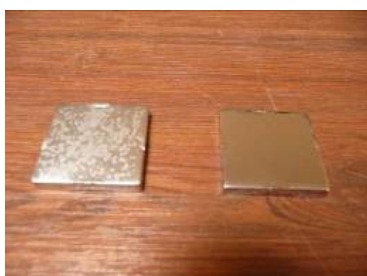
Fig. 4: A (left) and B samples after long EP experiments at 20 and 5V. Sample A is covered with yellow spots.
