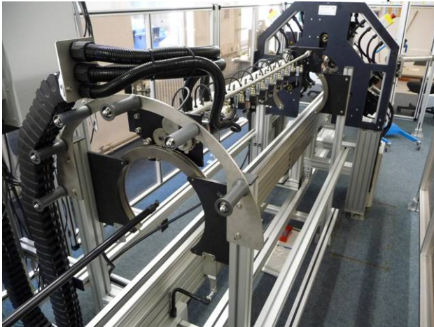
Figure 4: Eccentricity Measurement Device, showing the rotatable arm with the distance generators.
