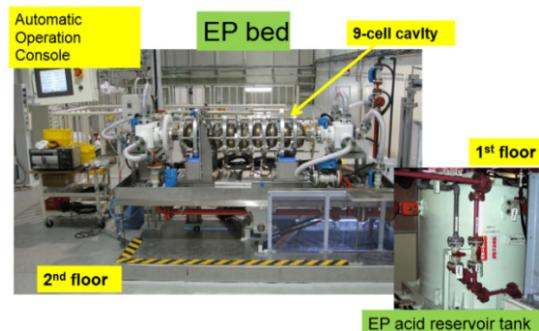
Figure 1: Pictures of the EP facility at STF/KEK. There is an EP bed on the 2<sup>nd</sup> floor and the reservoir tank of EP acid is on the 1<sup>st</sup> floor.
