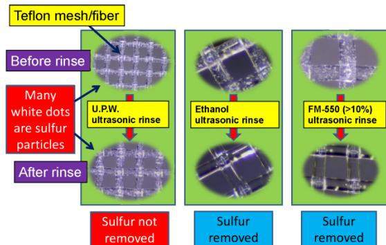
Figure 9: Some examples of test results. UPW rinse with ultrasonic vibration had almost no effect to remove sulfur particles on the Teflon-mesh sheet. Ethanol-rinse with ultrasonic vibration and FM-550 (>10%) with ultrasonic vibration removed all of sulfur particles on the Teflon-mesh sheet.
