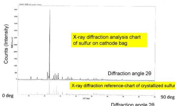
Figure 4: The analysis of ethanol and powder by X-Ray diffraction analyzer. Upper chart is for the powder and the lower chart is for the crystallized standard sulfur-sample.
