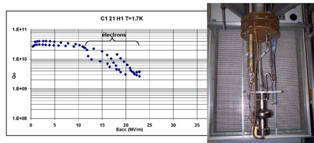
Figure 12: Left-hand side: The result of last vertical test for the single-cell cavity (C1-21) at CEA/Saclay. The  $Q_0$  vs.  $E_{acc}$  plot shows that the performance of the cavity is limited by field emission above the gradient of 10 MV/m. Right-hand side: The picture of vertical test stand for a single-cell cavity at CEA/Saclay.
