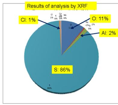
Figure 3: The analysis of ethanol and powder by X-Ray Fluorescence (XRF) analyzer. The main component of powder was found to be sulfur (86%). The rest of components were O (11%), Al (2%) and Cl (1%).
