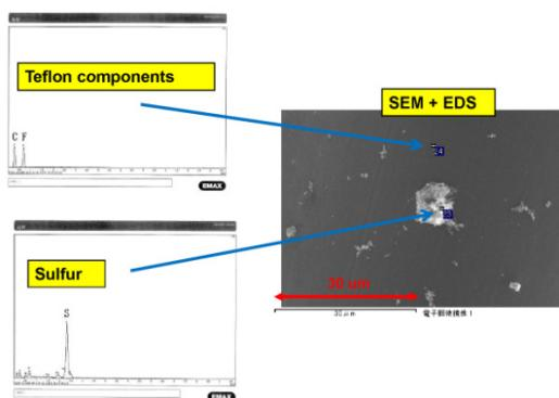
Figure 7: The results of EDS analysis for a particle on the surface of Teflon-mesh fiber. Lower left is EDS analysis on a particle and upper left is EDS analysis off the particle. The main component observed on the particle was sulfur. On the other hand, the main components observed off the particle were C and F which are the components of Teflon fiber.
