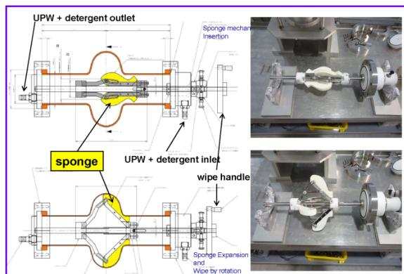
Figure 11: Left-hand side: the drawings of the proto-type sponge-wipe tool. Right-hand side: The pictures of the proto-type sponge-wipe tool.
