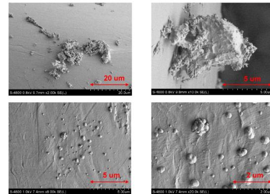
Figure 6: Images of particles on the detachable Teflon-mesh sheet by SEM.
