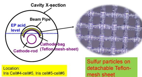
Figure 5: Left-hand side: The cross-section of cavity during EP process. Over the cathode-bag, detachable Teflon-mesh sheets were set in order to collect sulfur powder. Right-hand side: The picture of a detachable Teflon-mesh sheet by a microscope. Many particles of powder are seen as white dots on the surface of Teflon-mesh fibers.
