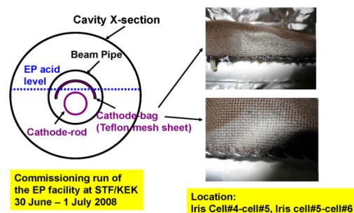
Figure 2: Left-hand side: The cross-section of cavity to illustrate the cathode-rod and the cathode-bag. Right-hand side: Pictures of the cathode-bag and the yellowish-white powder on it.
