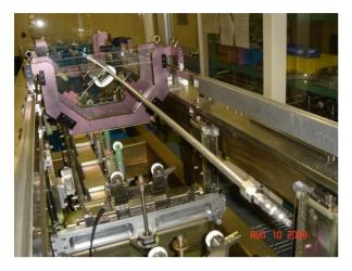
Figure 2: Long nozzle for HHPR guided by rails.
