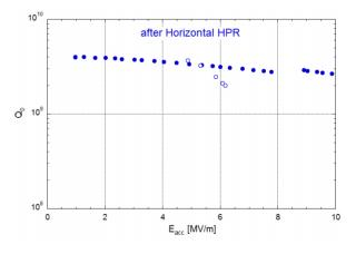
Figure 5: Q-E<sub>acc</sub> curve measured after HHPR
