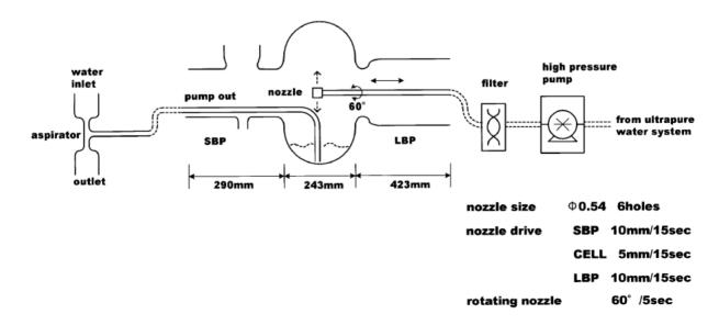
Figure 1: Conceptual design of horizontal high pressure water rinsing system.
