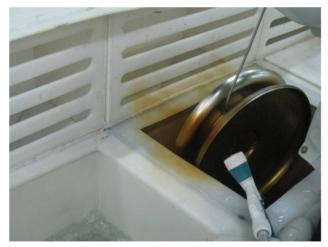
Figure 6: Etching before the electron beam welding.
