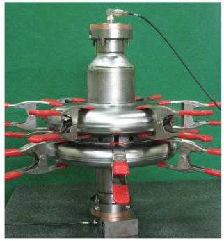
Figure 8: Frequency measurement set-up.
