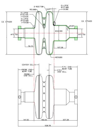
Figure 1: Drawing of the two-cell cavity.
