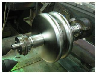
Figure 7: Cavity mounted on the electron beam welder.
