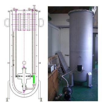
Figure 14: Cryostat for the vertical test.
