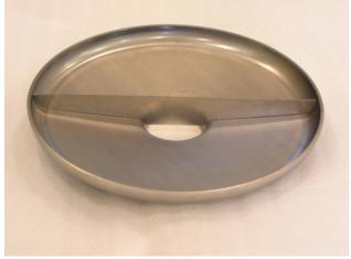
Figure 3: Half-cell after deep drawing.
