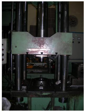
Figure 2: Deep drawing process to make a half-cell.
