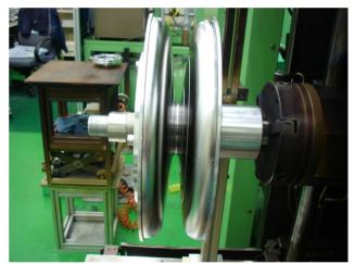
Figure 4: Dumbbell fabrication by joining two half cells by using the electron beam welding.
