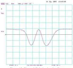
Figure 12: Phase shift during bead-pull test.
