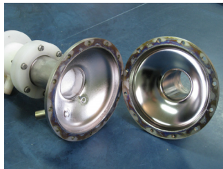
Figure 10: The picture of demountable cavity after BEP.
