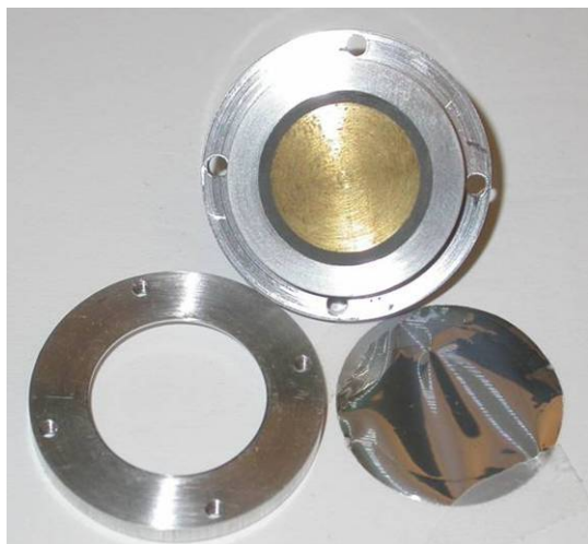
Figure 3: The oscillating superleak transducer components are shown: in the middle the isolated electrode with the sensor body, lower right the filter membrane and lower left the assembly ring.
