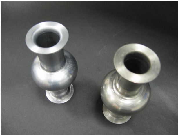
Figure 4: On the right a scrap, of a large Nb cavity, from which are obtained 4 small 6 GHz resonators from the 4 corners.
