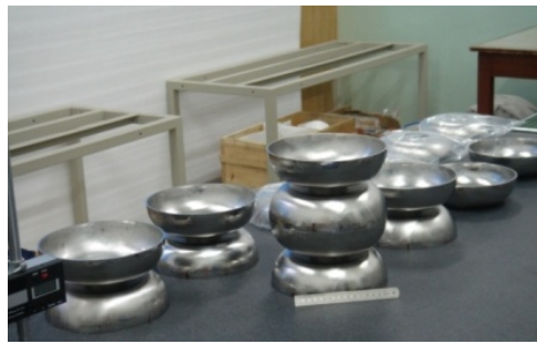
Figure 2: Half cells and dumbbells of the IHEP large grain 9-cell cavity
