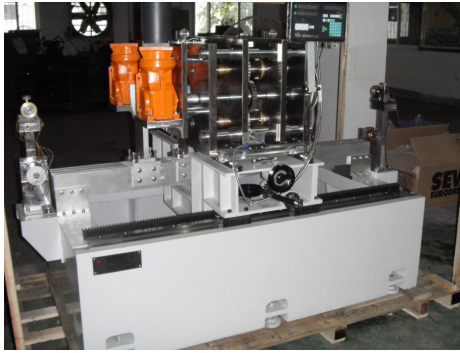
Figure 11: Pretuning machine for the 9-cell cavity. Longitudinal precision 2 \mu\text{m} , maximum force 10 kN (1000 kgf), maximum movement 6 mm.
