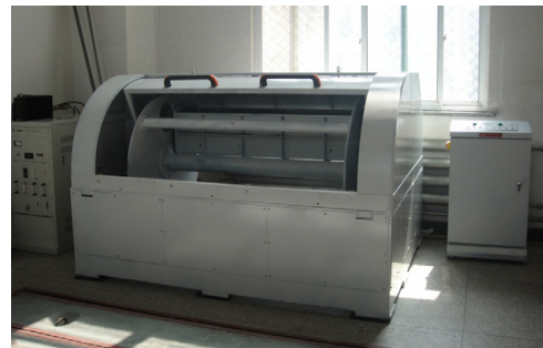
Figure 9: CBP machine for the 9-cell cavity. Normal rotating speed is 100 rpm.
